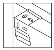
To mount the head rail, position it so that the front panel (A) rests at the top lip of the brackets. Then, push the bottom front of the head rail backwards and towards the window until the lip of the back of the head rail contacts the bracket and pops into place as shown in (B)
