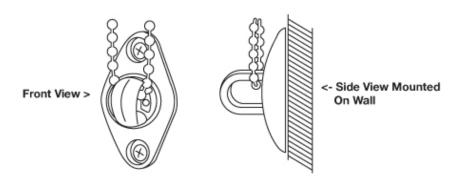
When installing the cord guide, make sure that the cord hangs loosely to optimize performance of the clutch and make sure that the cord connector passes through the guide with ease. Never twist or cross the control cord/bead chain, as this could damage the shade.
